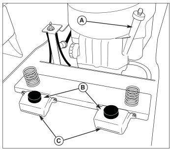
Figure 5. Checking the Fluid Levels
